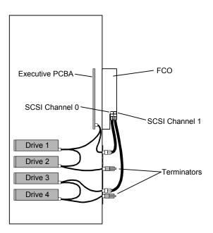
Figure 6-3 TLS-44xx Cabling Diagram
